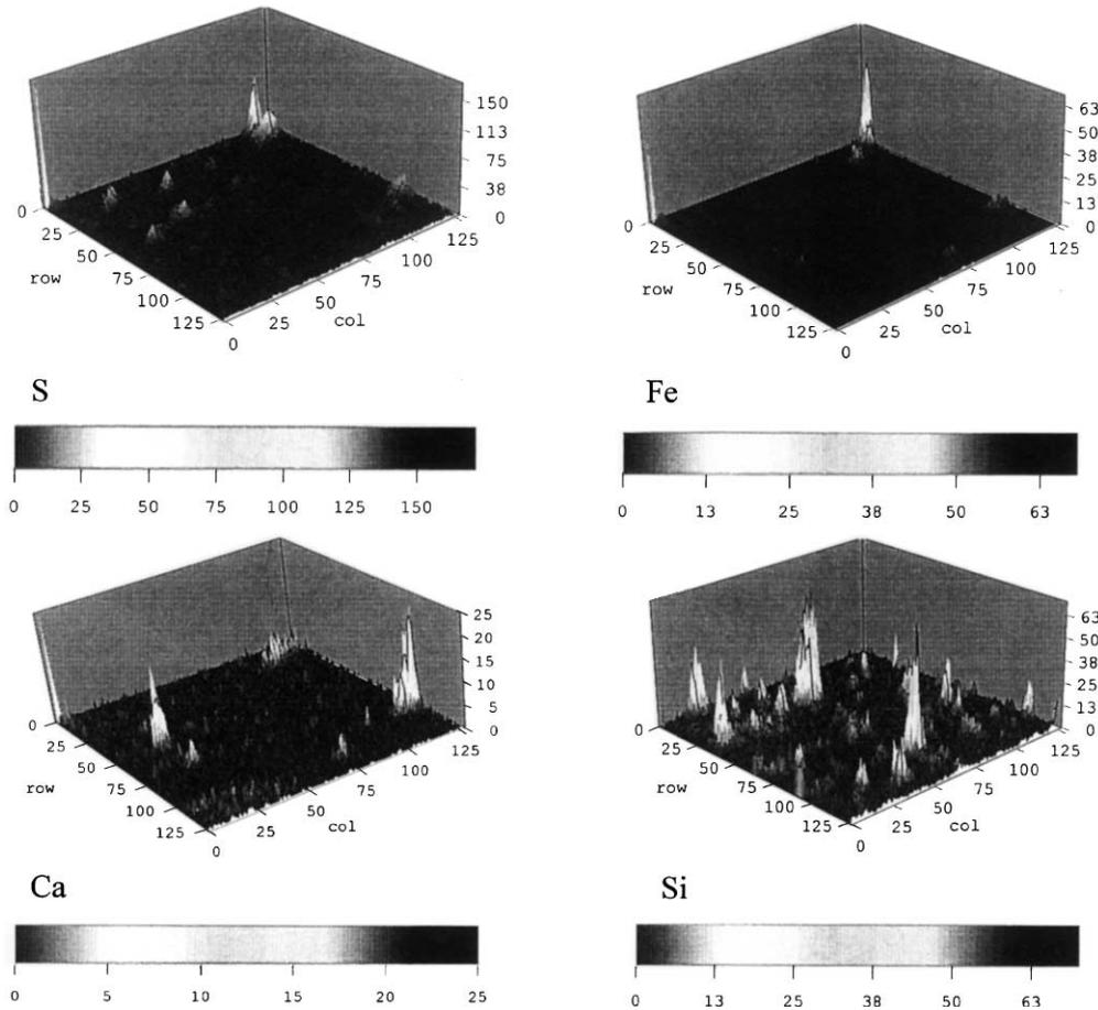
Fig. 6. Micro-PIXE elemental maps (scanning area = 25 μm × 25 μm) taken on the single Asian dust storm particles ( $\geq 1.2$  μm).
