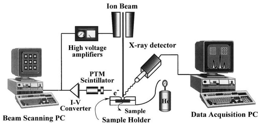
Fig. 2. Schematic diagram of the beam scanning and data acquisition system of micro-PIXE.
