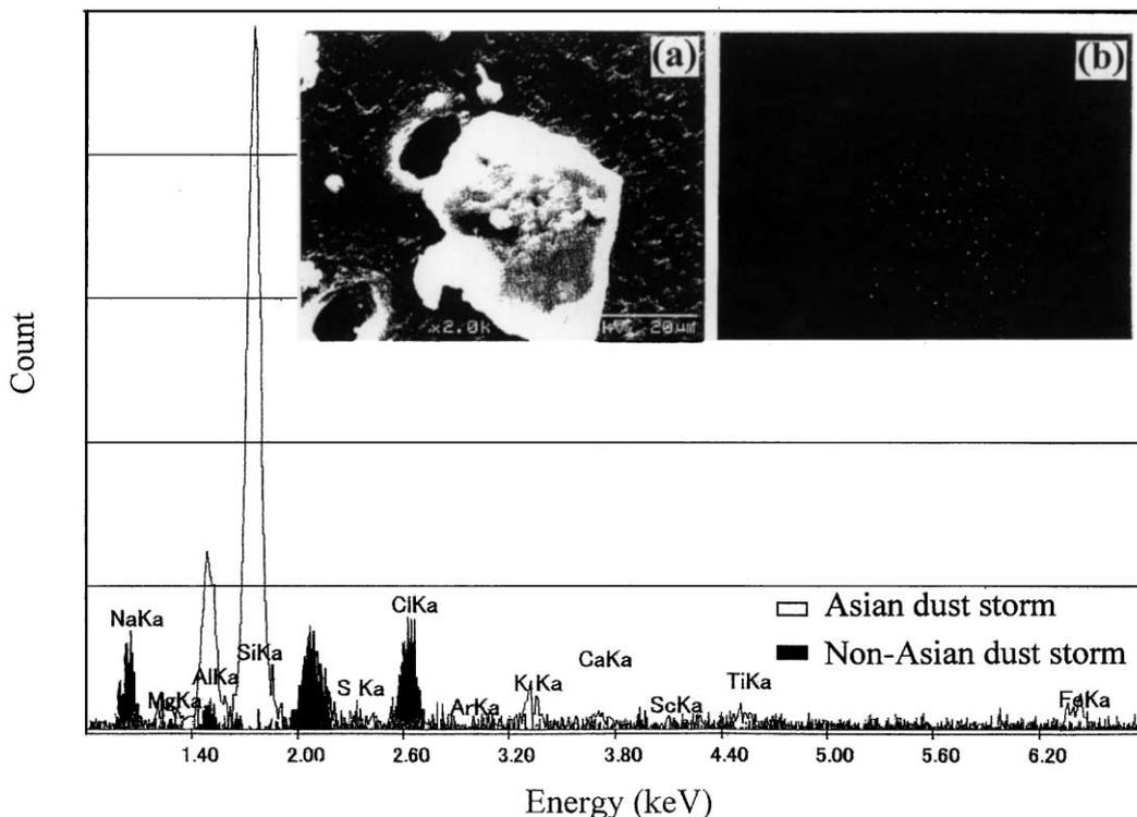
Fig. 3. X-ray spectrum, SEM image (a) and Si map (b) of single coarse particle collected in Asian dust storm event.
