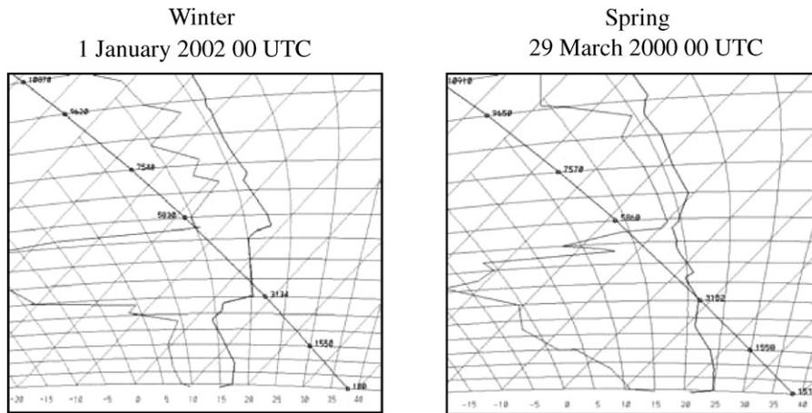
Fig. 5. Temperature profile showing low level inversion on most episode days.
